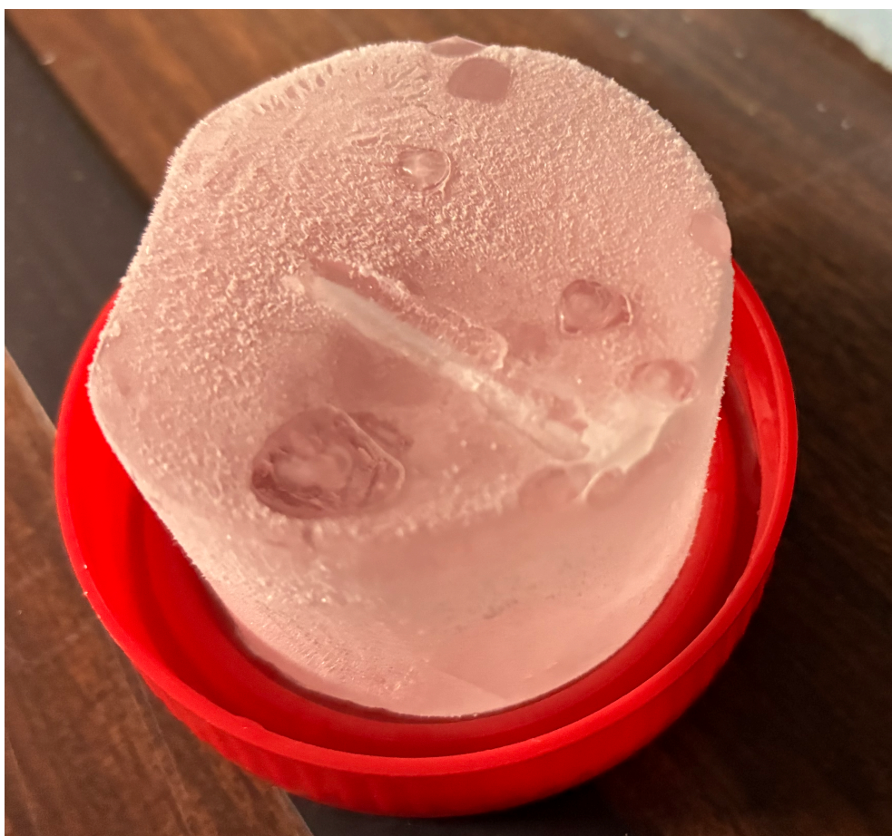
Visible damage of ice from thermal shock in prototype experiment
