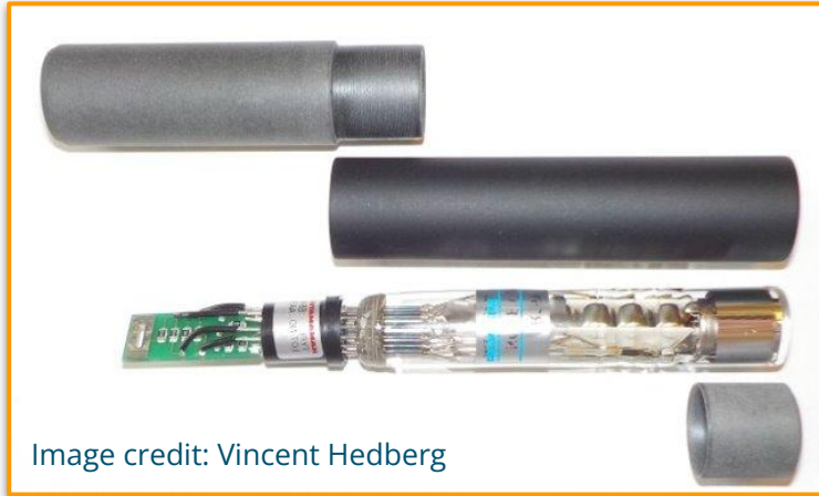
LUCID photomultiplier tube with shielding
