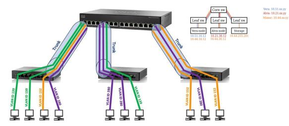
Traffic arriving on a switch port assigned to one VLAN will only ever be forwarded out another switch port that belongs to the same VLAN – **a switch will never allow traffic to cross a VLAN boundary**.
