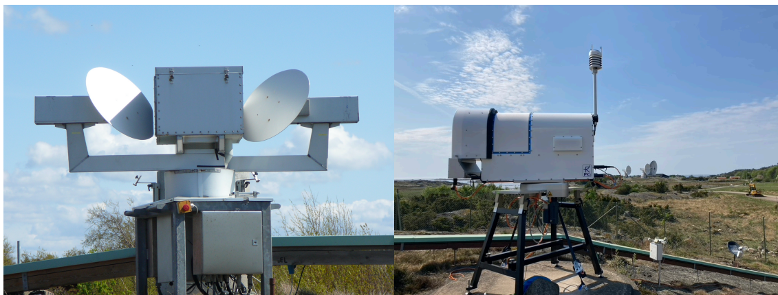
Figure 5: OSO's microwave radiometers to measure the amount of water vapor in the troposphere. Left: Konrad, operating since 1999. Right: Greta, installed in 2023.
